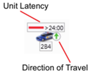
CAD Mapping – AVL unit showing latency bar.
